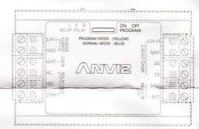
Switch in 'PROGRAM MODE' on the SC011: Move slide switch to left(ON).
